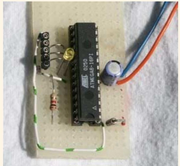
1 x ATmega8 DIP version, Atmel 8 bit Avr risc processor.
