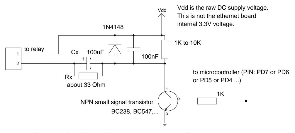
Cx and Rx are optional. They reduce the power consumption of the relay by a few milliampre. The exact value of Rx depends on the type of relay. Comon values are 22–68 Ohm. This circuit works because relays need a higher current when they switch and the current can be reduced when the contact just needs to be held.
